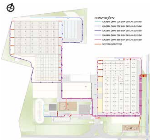
RAINWATER SEWER SYSTEM PLAN
